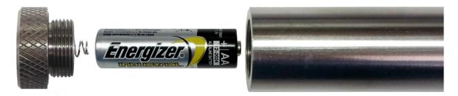
Ensure that all batteries are inserted into the chassis with the correct polarity. The negative terminal of the battery should be facing the bottom of the chassis. The positive terminal of the battery should be facing the antenna and the circuit board.
