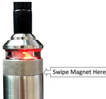
To turn the XMB-11K OFF using the magnet method, repeat the above procedure with the magnet swiped on the area below the antenna connection. Once the unit is turned off, it will no longer transmit a frequency.
