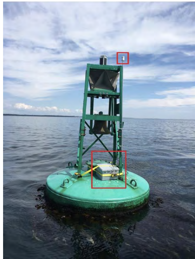
Fig. 2 - Brizo2 Deployment (Grey Box) on Navigation Bell Buoy in Herring Cove, NS. Antenna Above Buoy.
