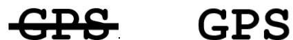
Pictured: Hermes GPS has not been updated, Hermes GPS has a current position
