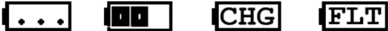
Pictured: Hermes battery before charge reading, partial charge, when charging, when a charging fault has occurred.
