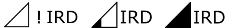
Pictured: Iridium Strength Bars; no signal, not registered, low signal, full signal
